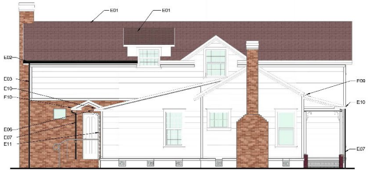
NORTH ELEVATION - MAIN HOUSE A1 1/4" = 1'-0"
