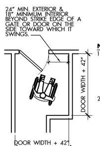
CLEAR SPACES MUST BE LEVEL TO PREVENT WHEELCHAIRS FROM ROLLING WHEN THE OCCUPANT RELEASES THE WHEEL GRIPS TO REACH FOR THE DOOR. 1/4" PER FOOT IS ALLOWED FOR DRAINAGE.
