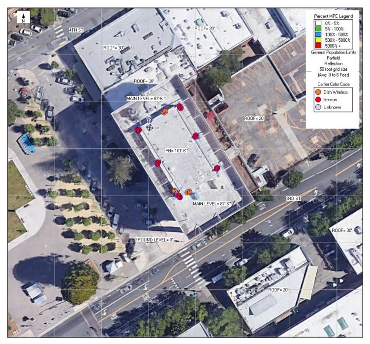
The reference plane for the plot is the Ground Level 0' (DISH Wireless Only).
