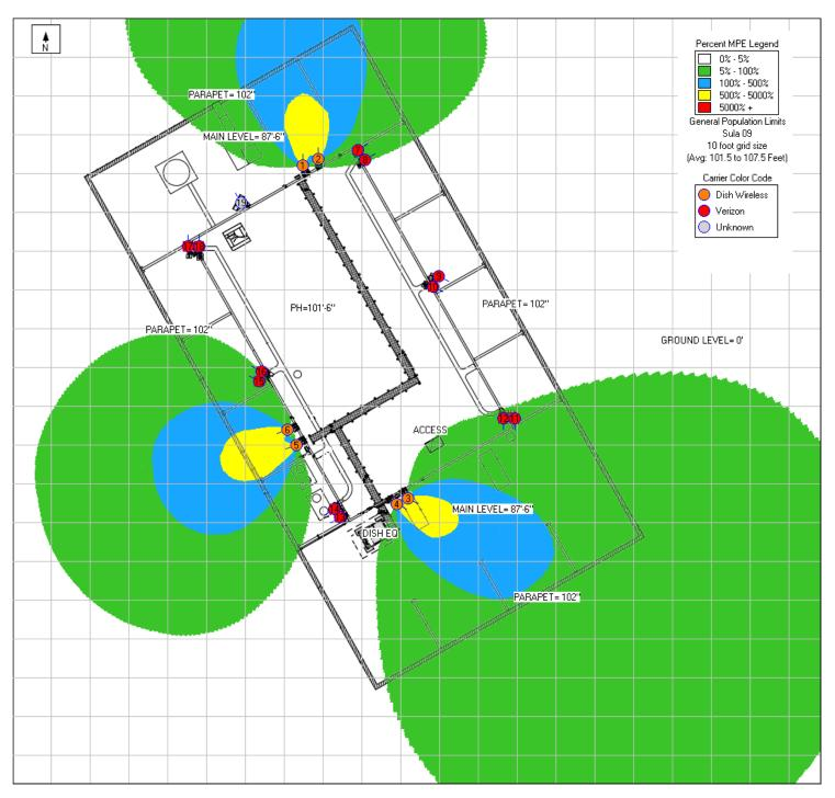
The reference plane for the plot is the Penthouse Level 101'-6" (DISH Wireless Only).
