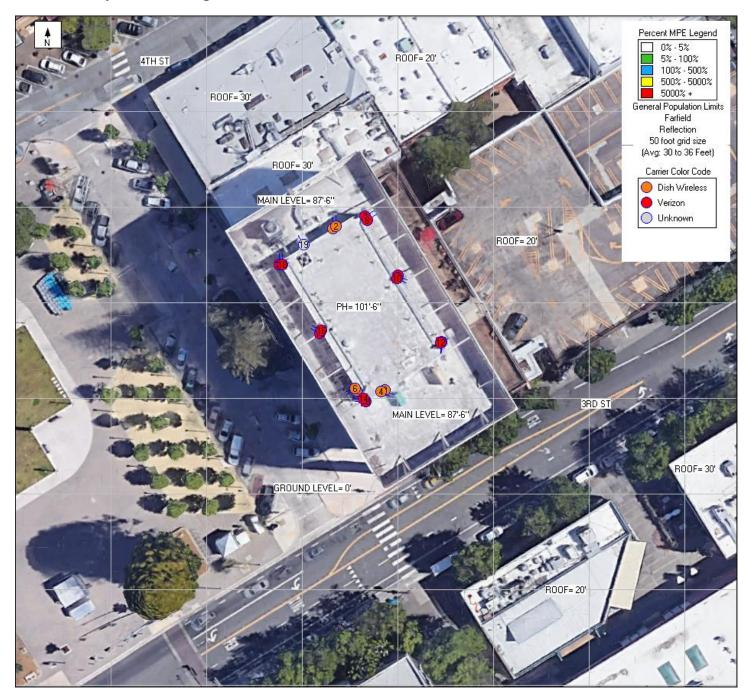
The reference plane for the plot is the Adjacent Building Level 30' (DISH Wireless Only).
