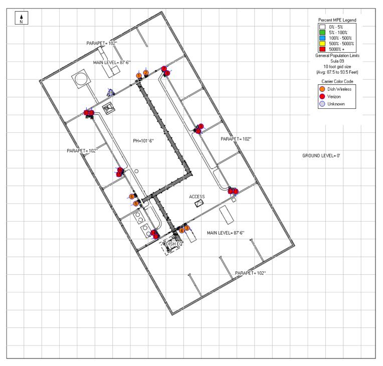
The reference plane for the plot is the Main Level 87'-6" (DISH Wireless Only).
