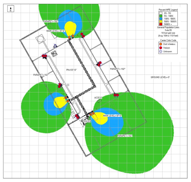
The reference plane for the plot is the Antenna Level 104' (DISH Wireless Only).
