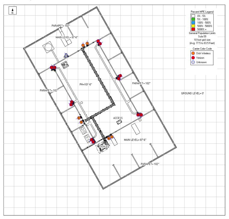
The reference plane for the plot is the Top Floor Level 77'-6" (DISH Wireless Only).
