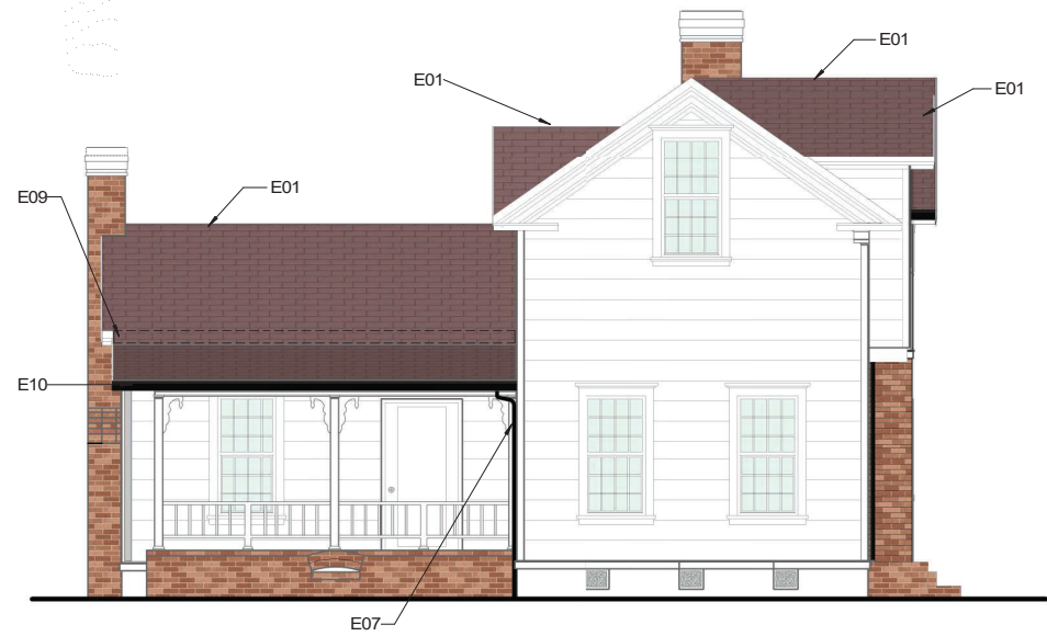
WEST ELEVATION - MAIN HOUSE C3 1/4" = 1'-0"
