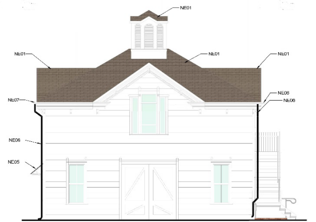
CARRIAGE HOUSE - NORTH ELEVATION A1 1/4" = 1'-0"
