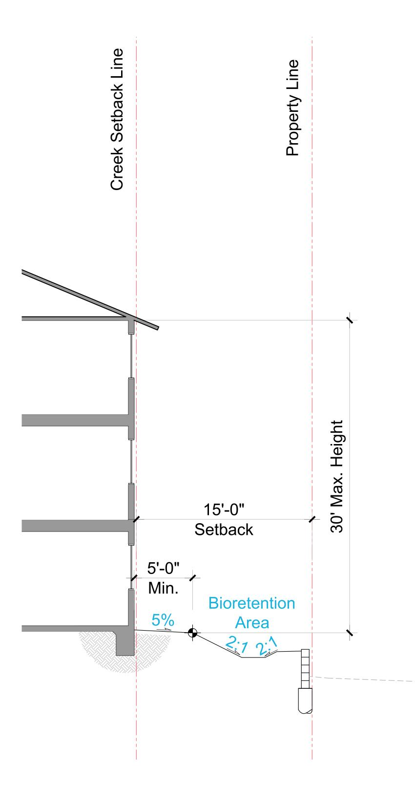
SECTION 'A-A' ROOF DESIGN CONDITION 1
