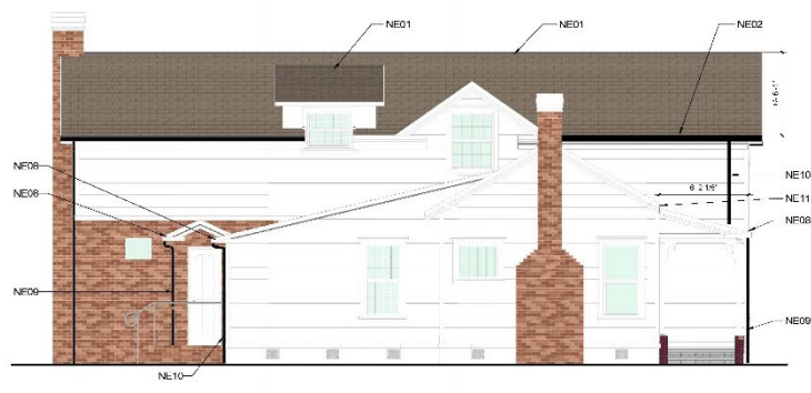
NORTH ELEVATION-MAIN HOUSE A1 NF=1-7'
