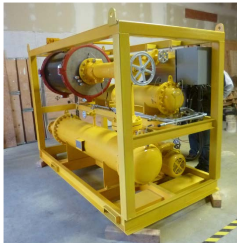
Figure 6-3: Infinity Turbine ORC
