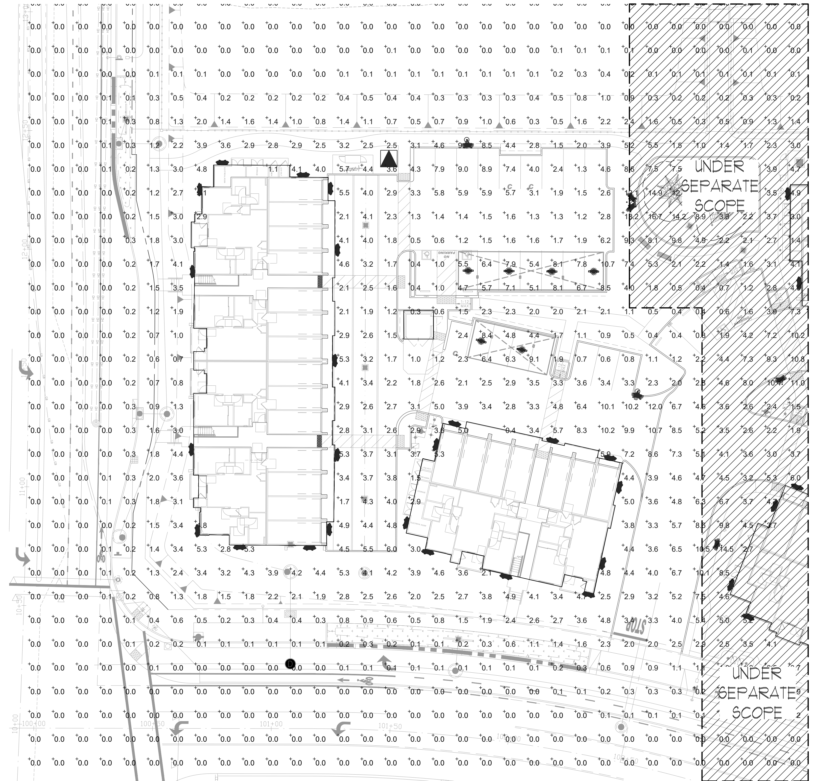
A PARTIAL SITE PHOTOMETRIC PLAN 1" = 20'-0"
