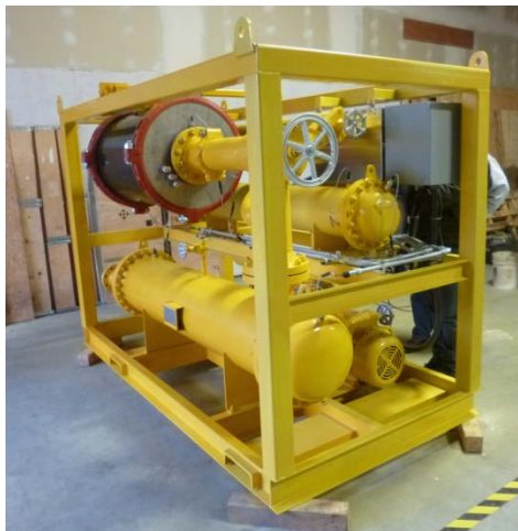
Figure 6-3: Infinity Turbine ORC
