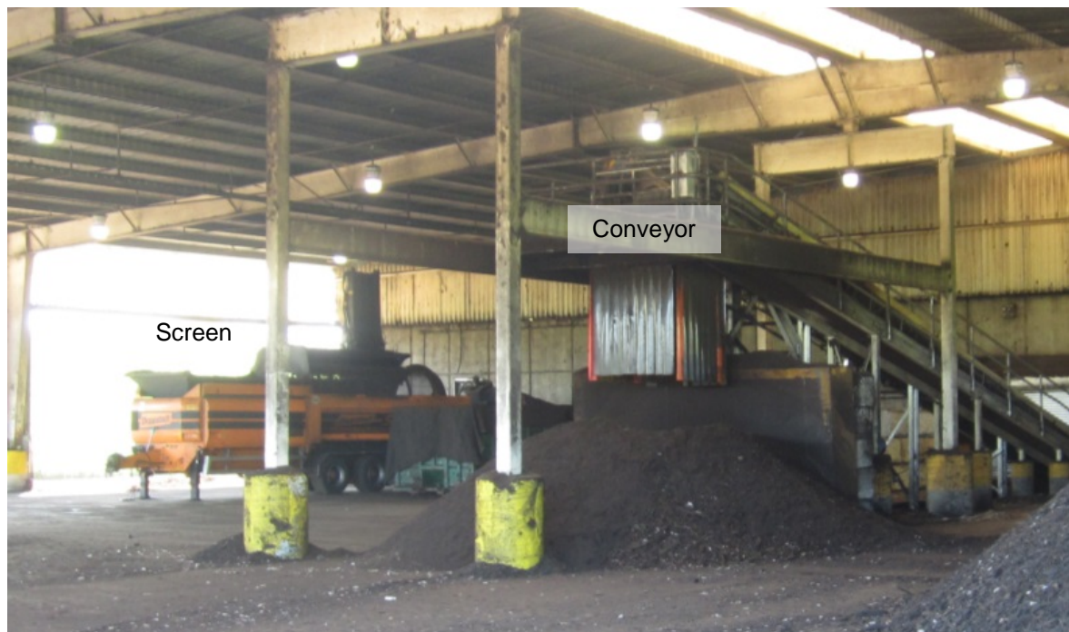
Figure 2-5: Screening Equipment Location Relative to Conveyor
