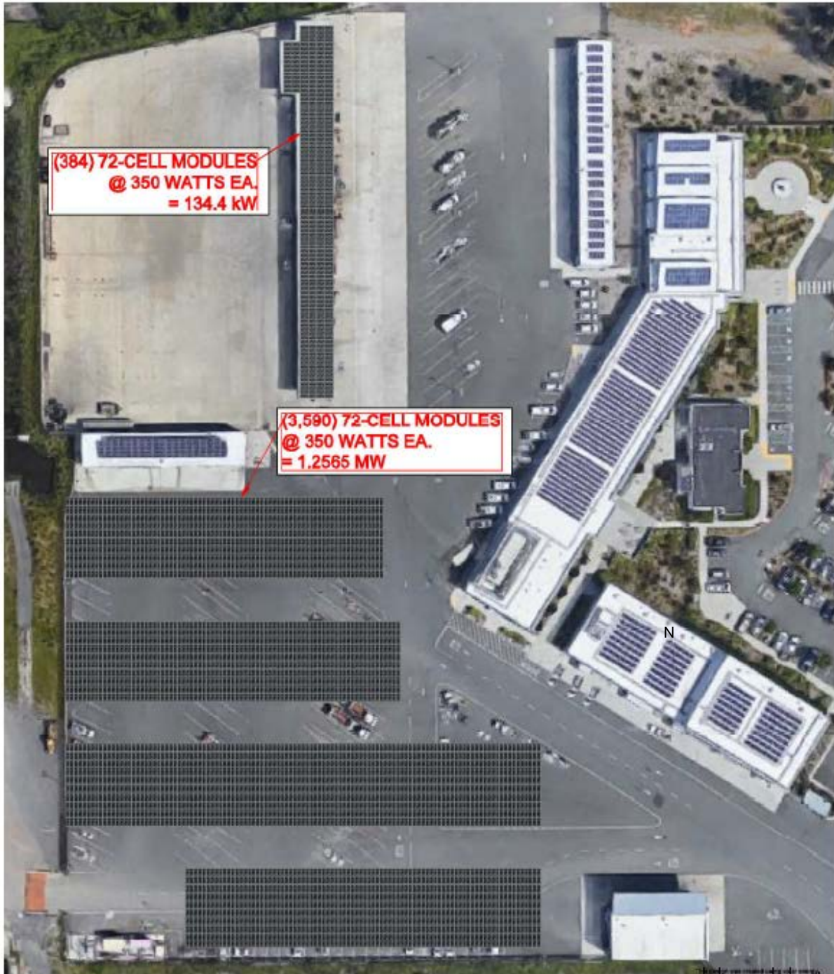
Figure 7-4: Solar PV Carport Layout
