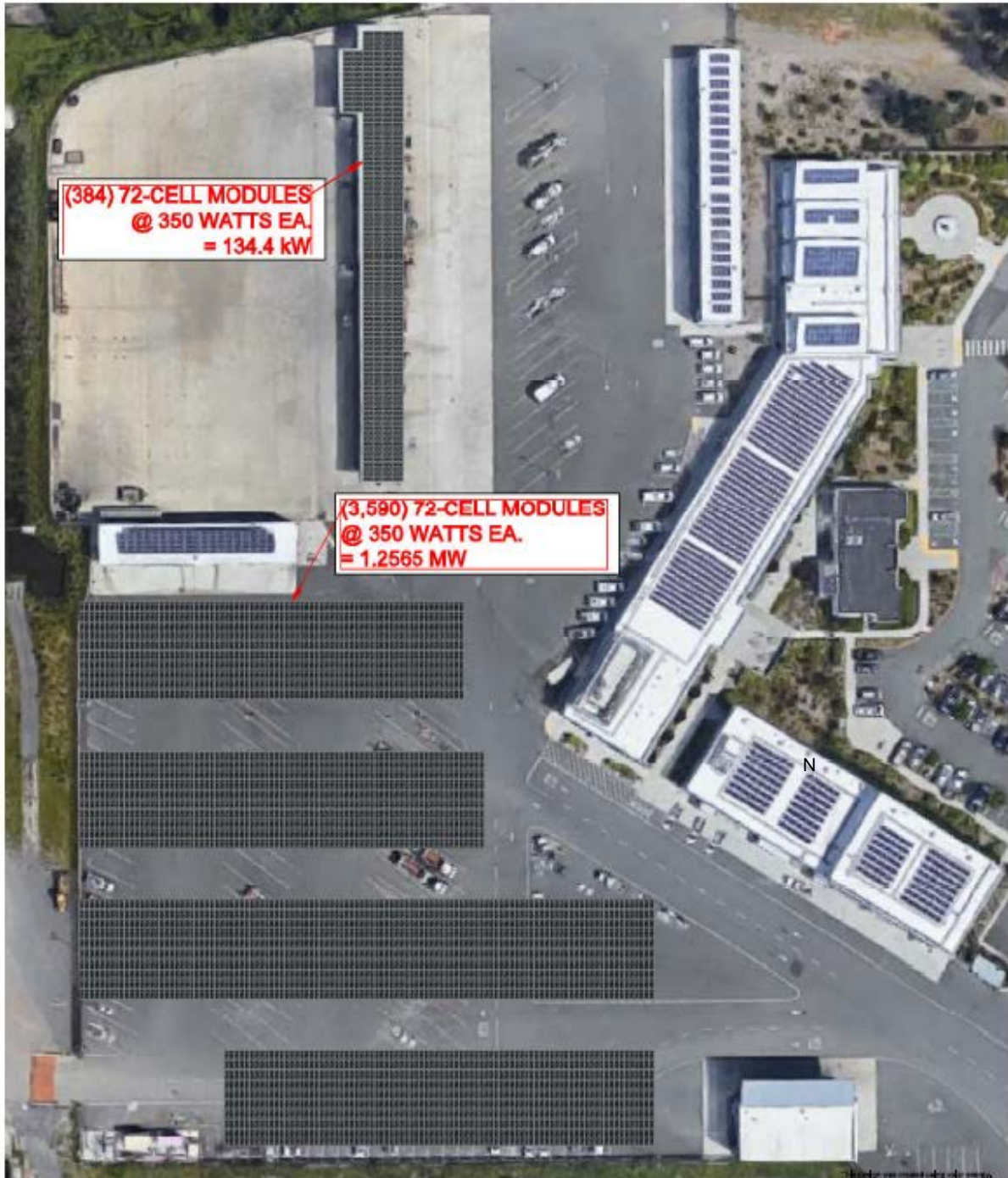
Figure 7-4: Solar PV Carport Layout
