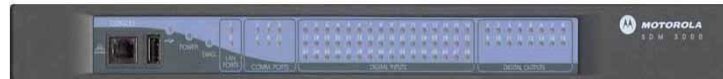
Figure 1-9: SDM3000 Remote Terminal Unit – Enables the UEM to acquire information regarding the fault and configuration of elements/devices in sites
