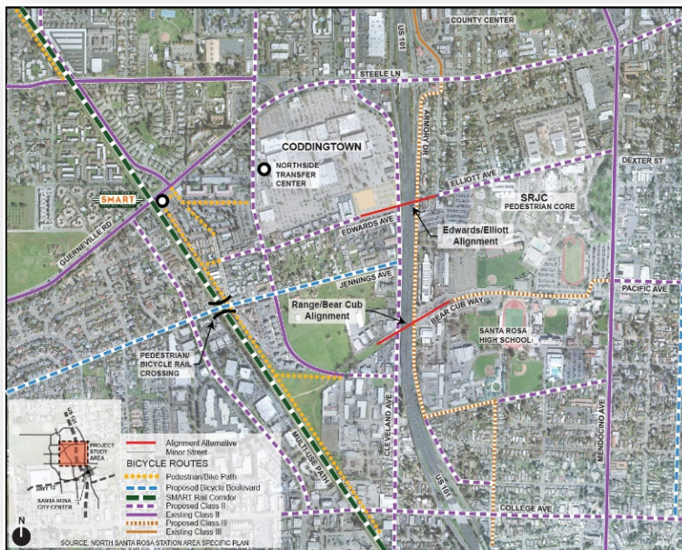
Highway 101 Bike and Pedestrian Bridge alignment options
