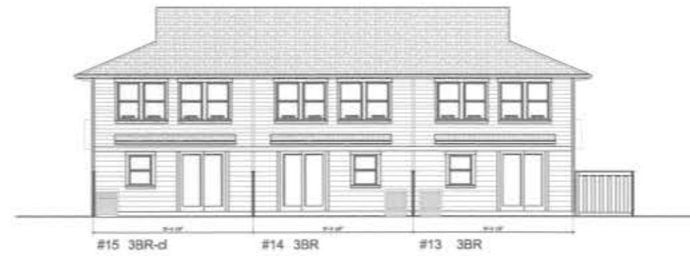
② Exterior Elevation - South Units 13-15 1/8"=1'-0"
