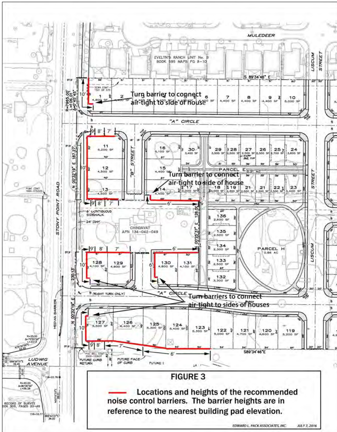
Figure XII-1: Noise Control Barriers Detail
