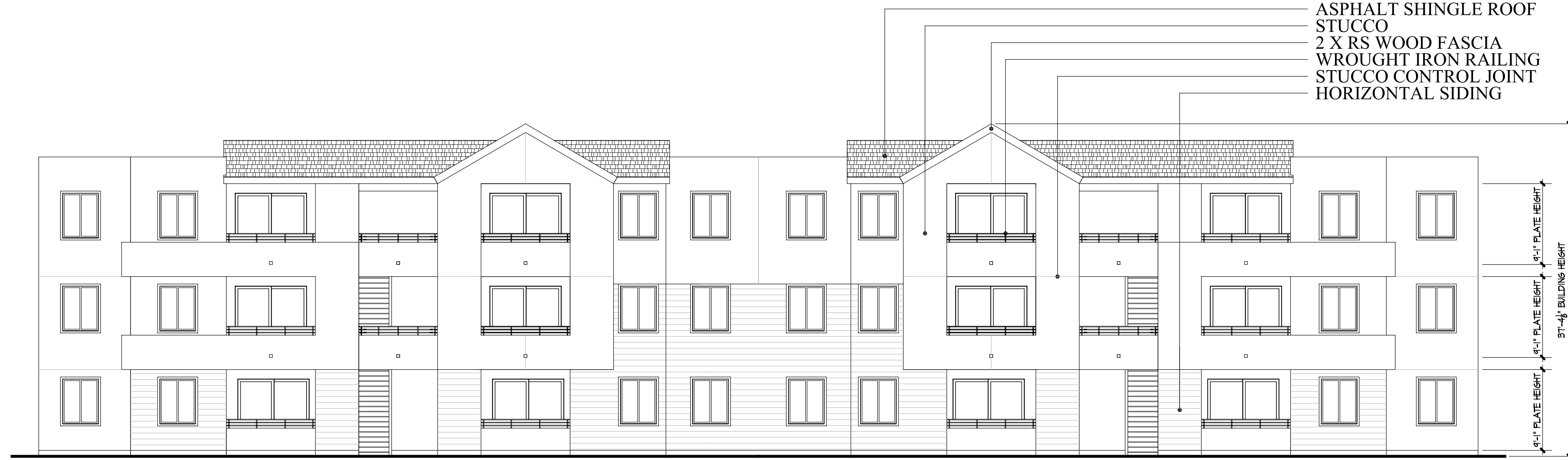
FRONT ELEVATION - BUILDING B
