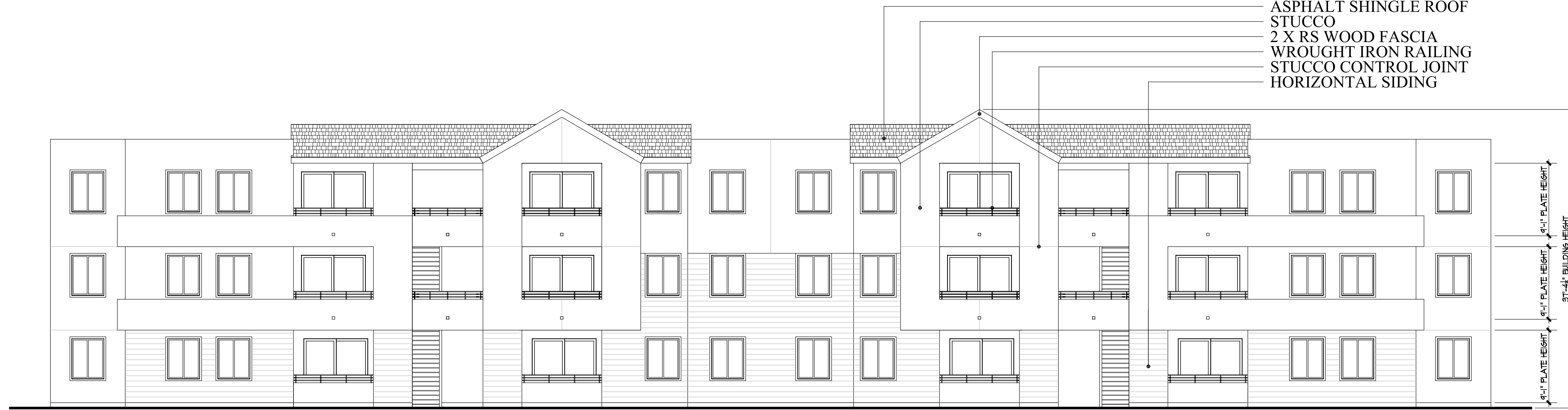
FRONT ELEVATION - BUILDING A
