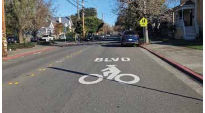
Class IIIB bike boulevard roadway marking on the Humboldt Street Bike Boulevard in Santa Rosa. The street also includes speed humps as traffic calming.
