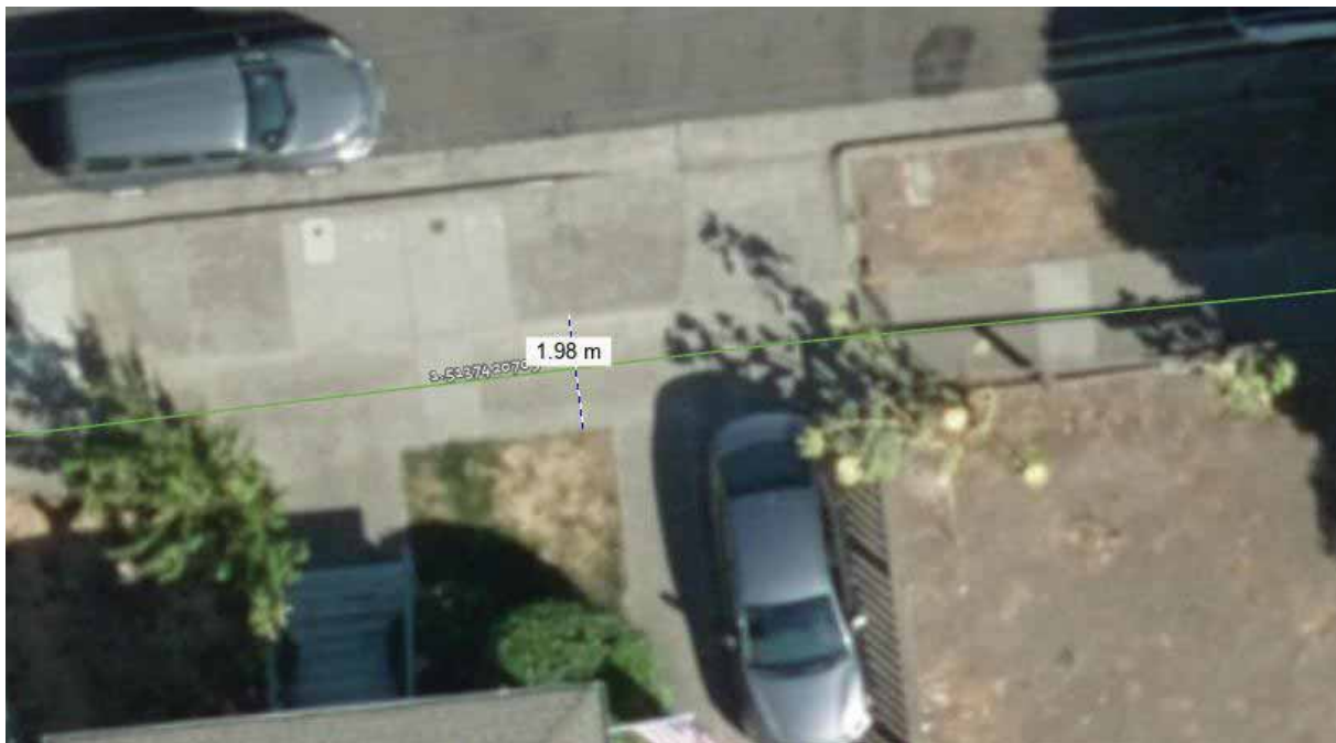
Figure 76. A discrepancy is shown between Ecopia-provided sidewalk width (shown in small white text, 1.5 m or 4.9 feet), and Alta-measured width, 1.96 m or 6.4 feet. This difference is equal to about one and a half feet.
