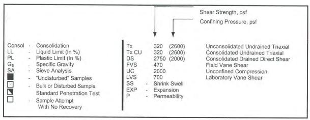
Note: All strength tests on 2.8" or 2.4" diameter sample unless otherwise indicated
