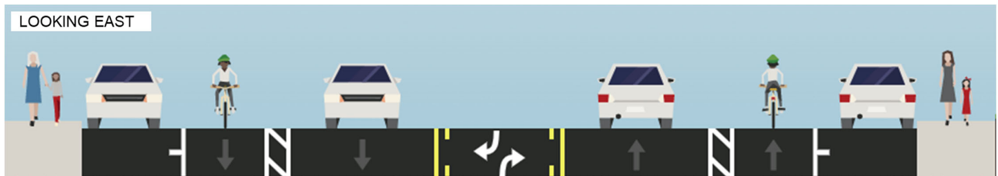
Figure 43 Proposed Improvements on 4th Street from Brookwood Ave to Bryden Ln (Cross Section View – Looking East)
