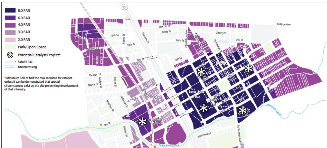
Figure 2: Downtown Station Area Specific Plan. This view of the Preferred Plan Concept overlays proposed Floor Area Ratio (FAR) maximums throughout the Plan area. FAR represents the amount of building area that can be developed on a parcel of land. The number preceding is the multiplier applied to the area of the parcel.
