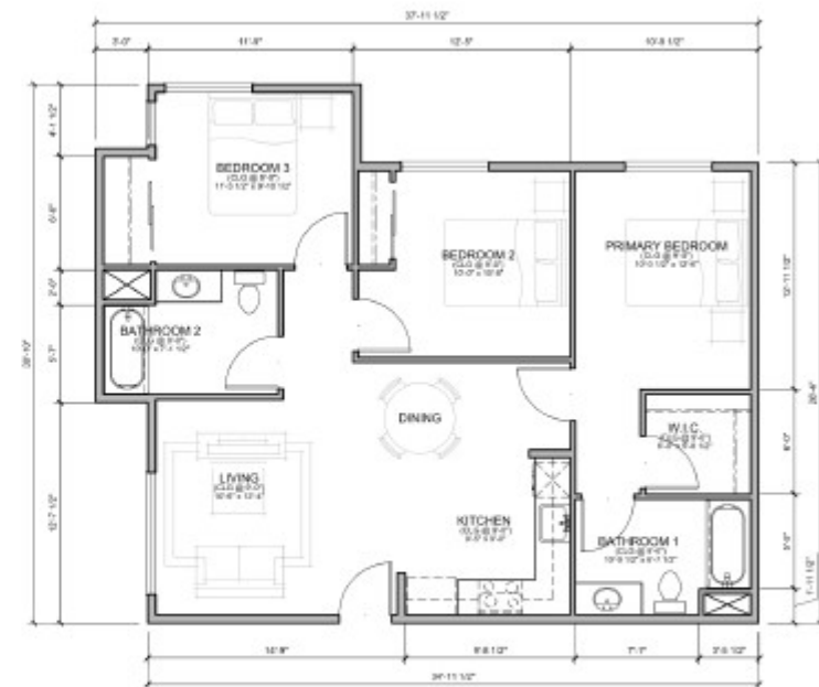
UNIT 3B - 3BED/2 BATH GROSS SF: 1019 SQ. FT. NET SF: 948 SQ. FT.
