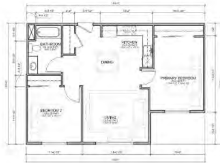
UNIT 2B - 2BED/1 BATH GROSS SF: 781 SQ. FT. NET SF: 729 SQ. FT.
