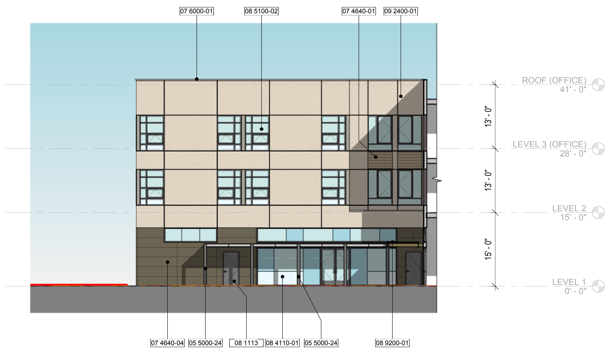
CARITAS CENTER - WEST ELEVATION - INTERIOR ④ 1" = 10'-0"
