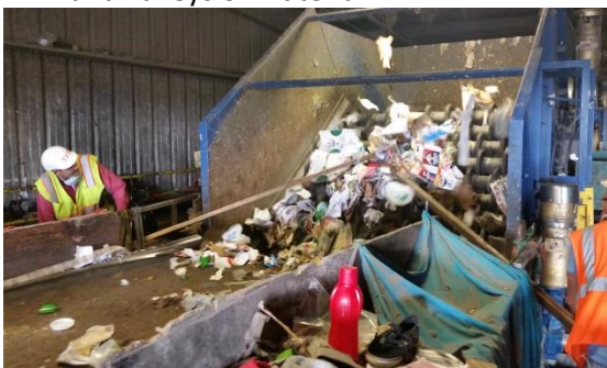
4) Workers pushing materials up Star Screen with 2x4 beams – (likely OSHA violation)
