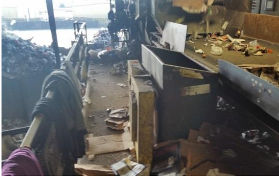
1) Poor MRF Housekeeping; Chain Guard Removed and Posing a hazard – (likely OSHA violations)
