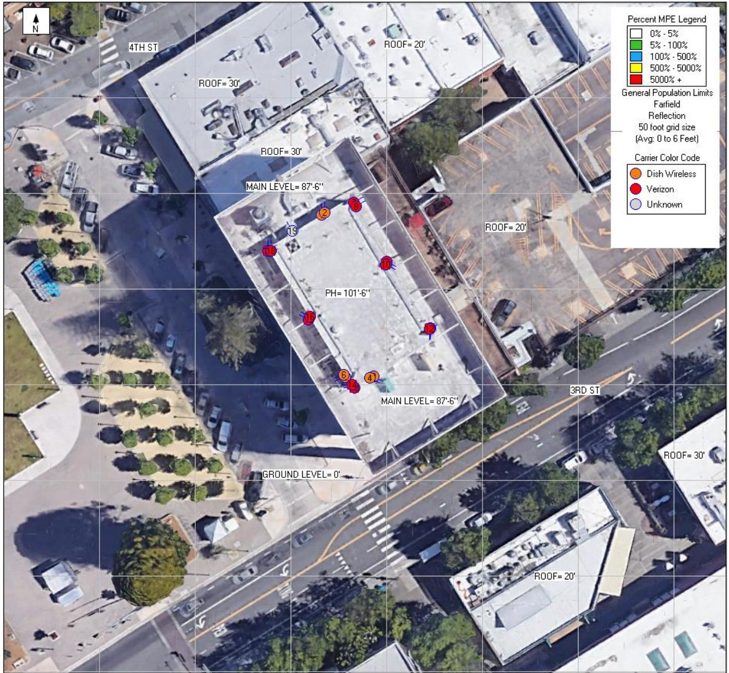
The reference plane for the plot is the Ground Level 0' (DISH Wireless Only).
