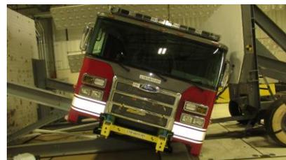
**Frontal Impact:** The test cab was struck by the 14,320 lb. moving barrier at a speed sufficient to impart the required 65,098 ft-lbs. of energy. Twice the energy required per SAE J2420.
