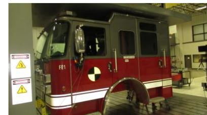
Pass-Fail criteria of the SAE tests and the ECE 29 test is a measure of whether the “survival space” inside the cab is compromised, all doors remain shut, and the cab remained attached to the chassis frame in at least one location. The Pierce cab met all of the Performance Criteria requirements on all 3 integrity tests.
