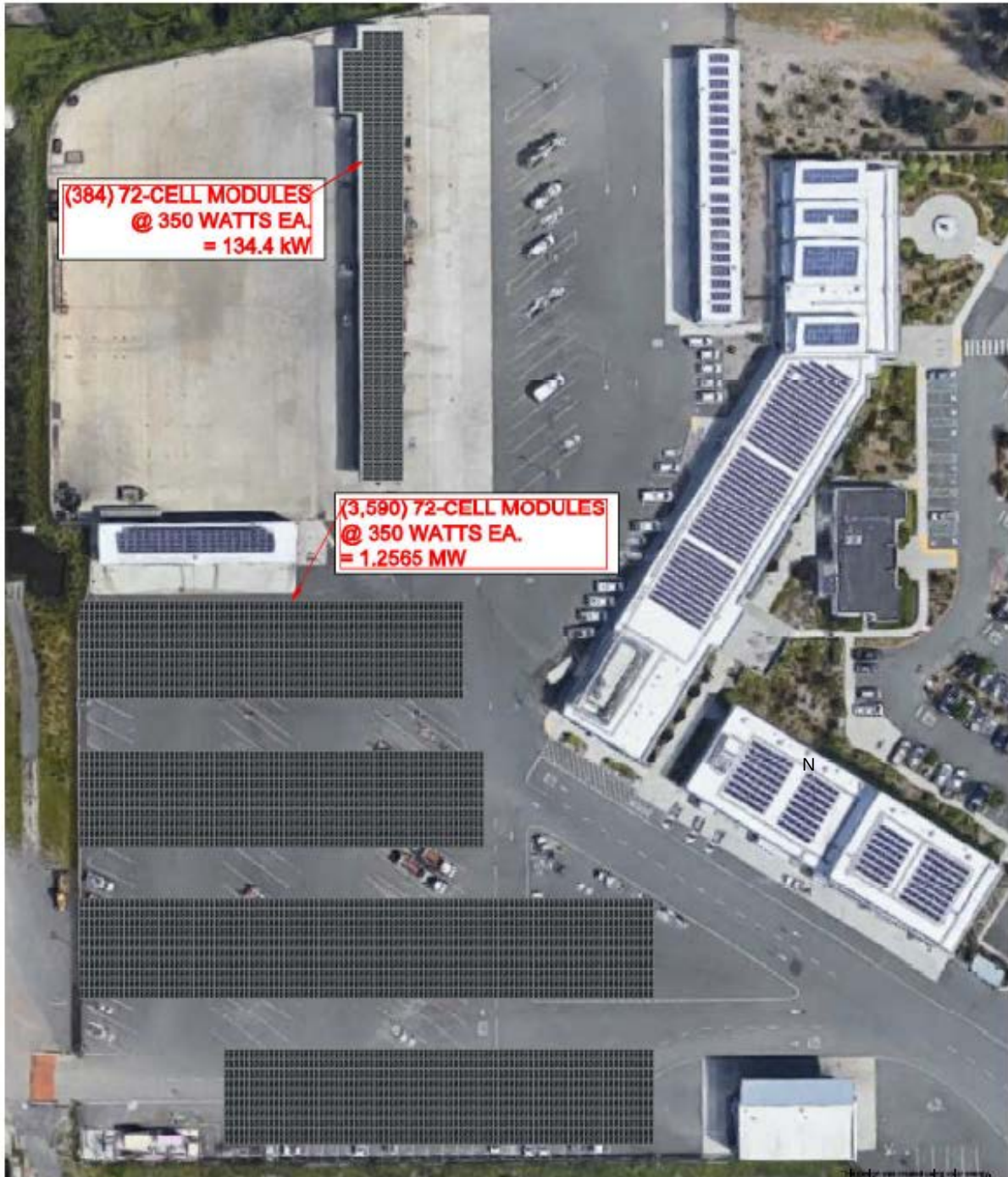
Figure 7-4: Solar PV Carport Layout
