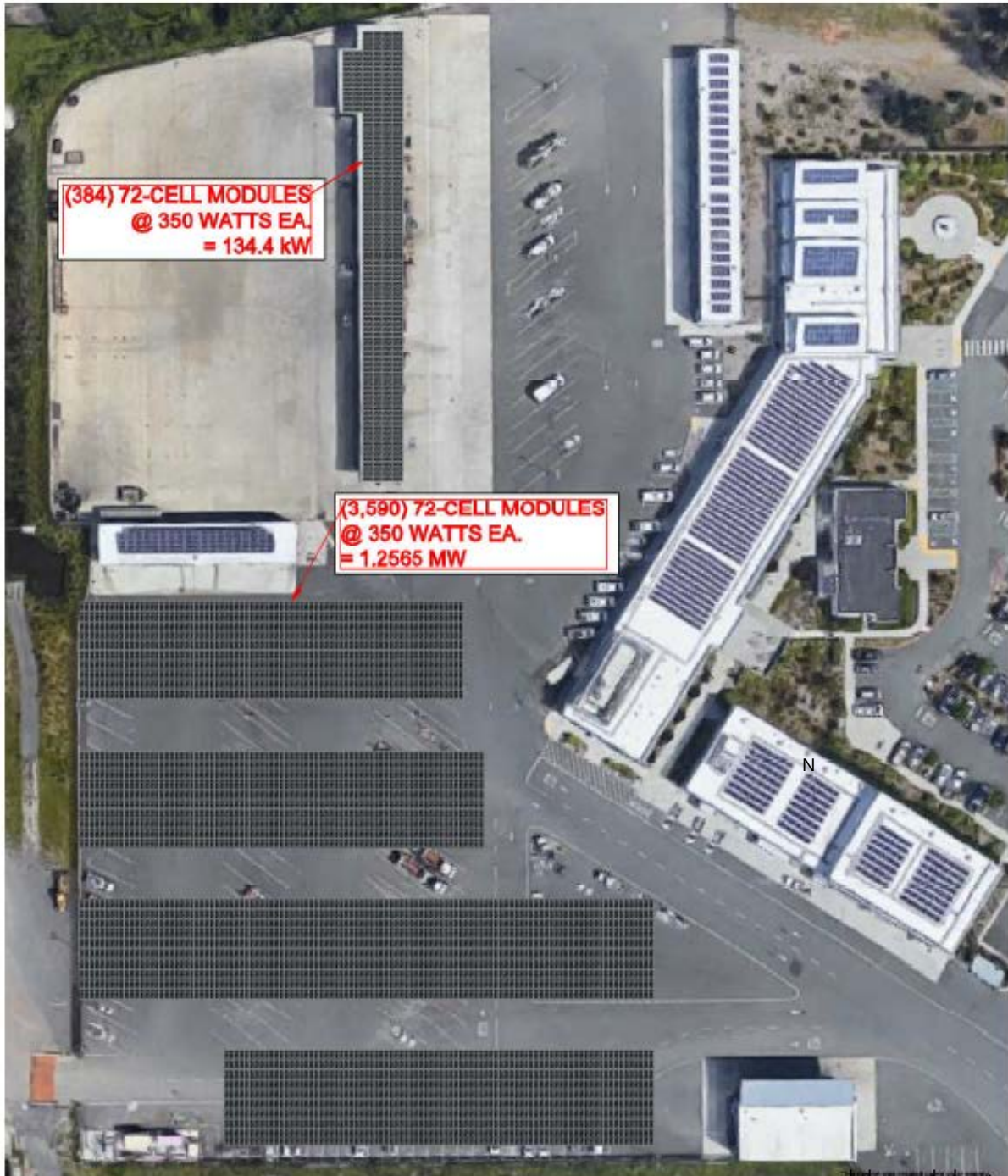
Figure 7-4: Solar PV Carport Layout
