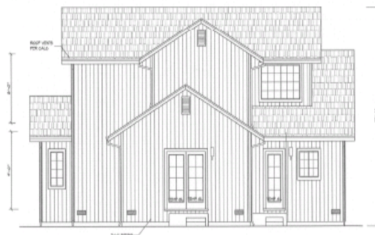
REAR ELEVATION LOT 1 SCALE 1/4"=1'-0"
