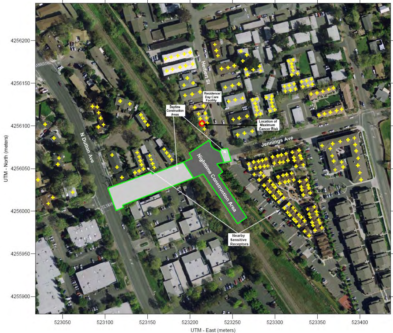
Figure 2. Over-Crossing Construction Areas, Residential Receptors, and Location of Maximum Cancer Risk and PM 2.5
