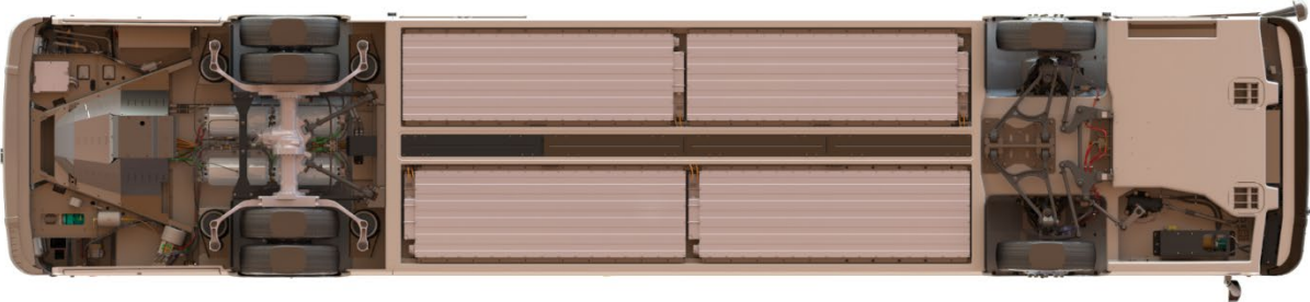
Figure 1 Locations of HV Battery Packs for ZX5 + Configuration (4 packs)
