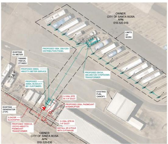
**Note:** per Customer's request after the Prelim Deigns was completed, customer's meter service and Distribution Panel will be moved South/East about 10' in the Final Design Stage if possible.
