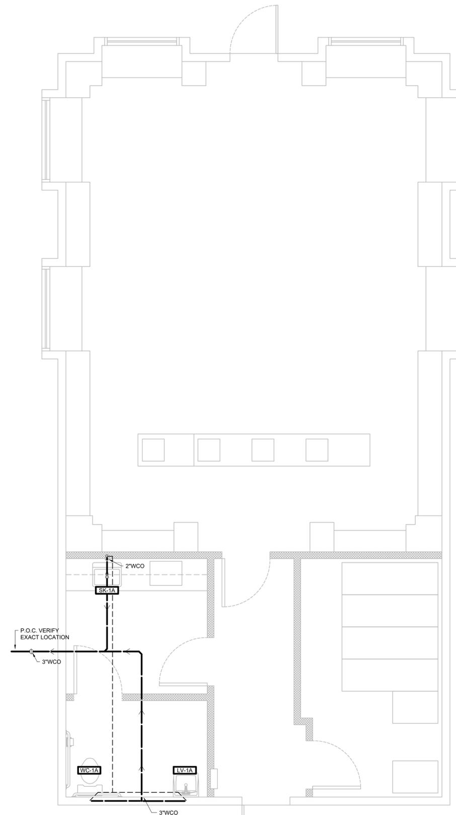
PLUMBING FLOOR PLAN WASTE & VENT
