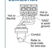
**ATTENTION:** Unit must be hard wired. NOTE: Heater is single phase. All tests are measured at the output of the heater.
