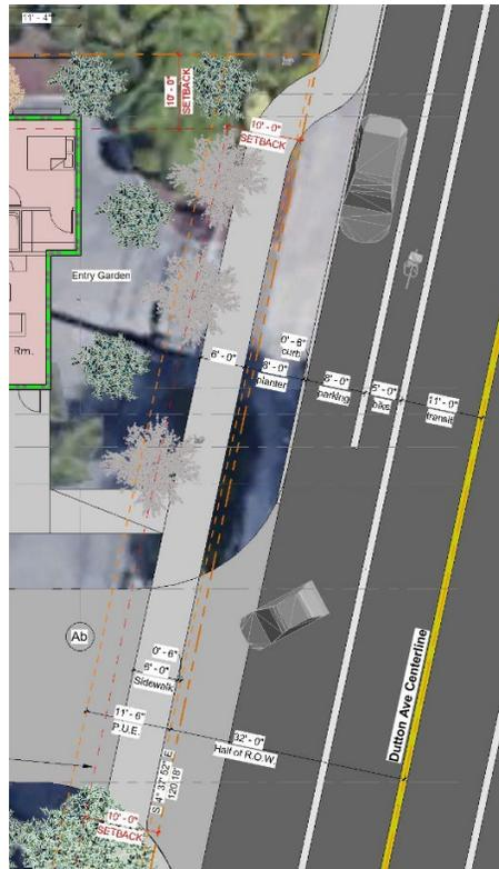
Figure 6 – Right of Way Widening on Dutton Avenue
