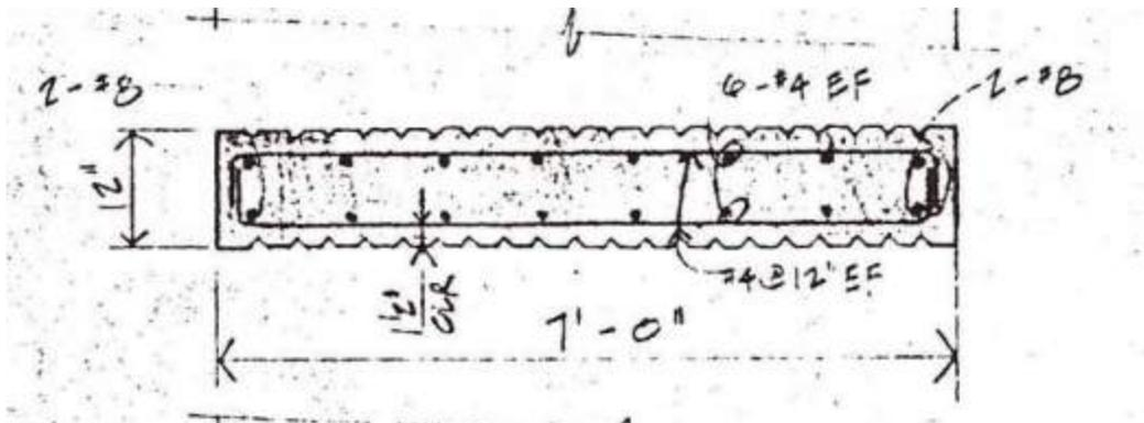
Figure 26: Building 11 Concrete Shear Wall Section
