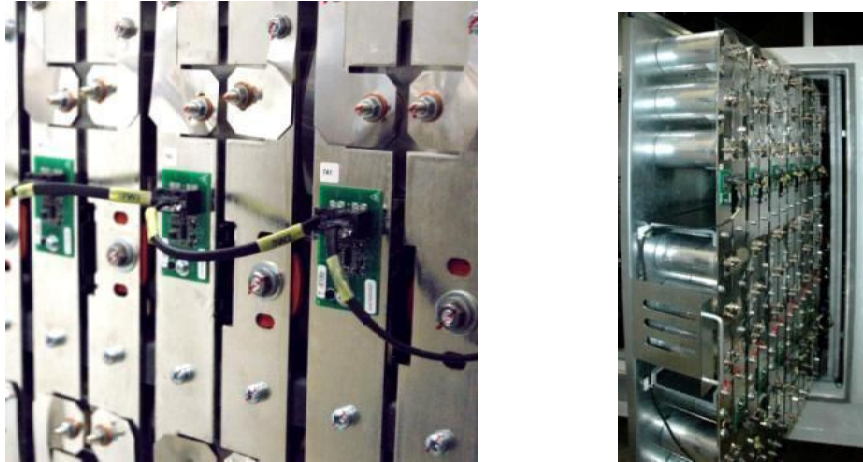
Figure 4: Temperature sensors are on all critical components and on the bus bar.
