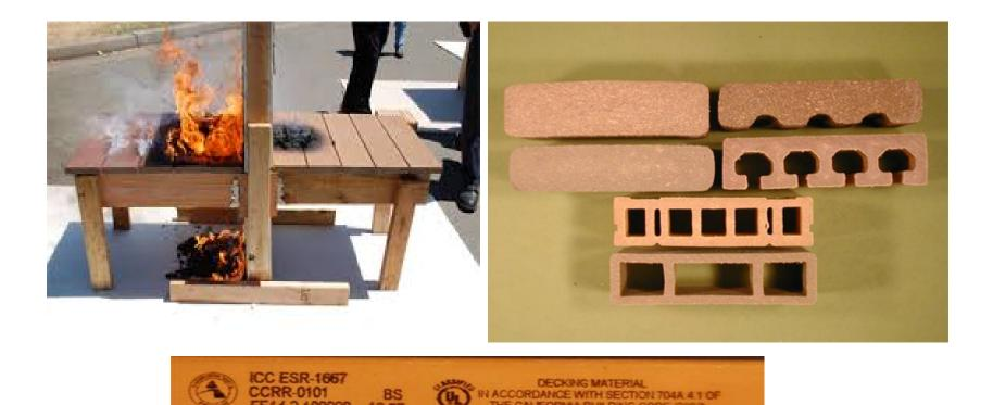
**Decking Material and Floor Projection requirements** – when located within 10 feet of the building the materials shall meet specific testing criteria as outlined in Chapter 7A or the SFM Standards 12-7A-4A.
