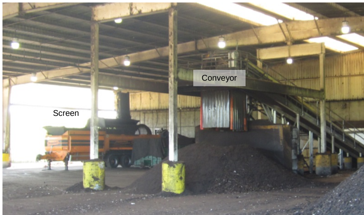
Figure 2-5: Screening Equipment Location Relative to Conveyor
