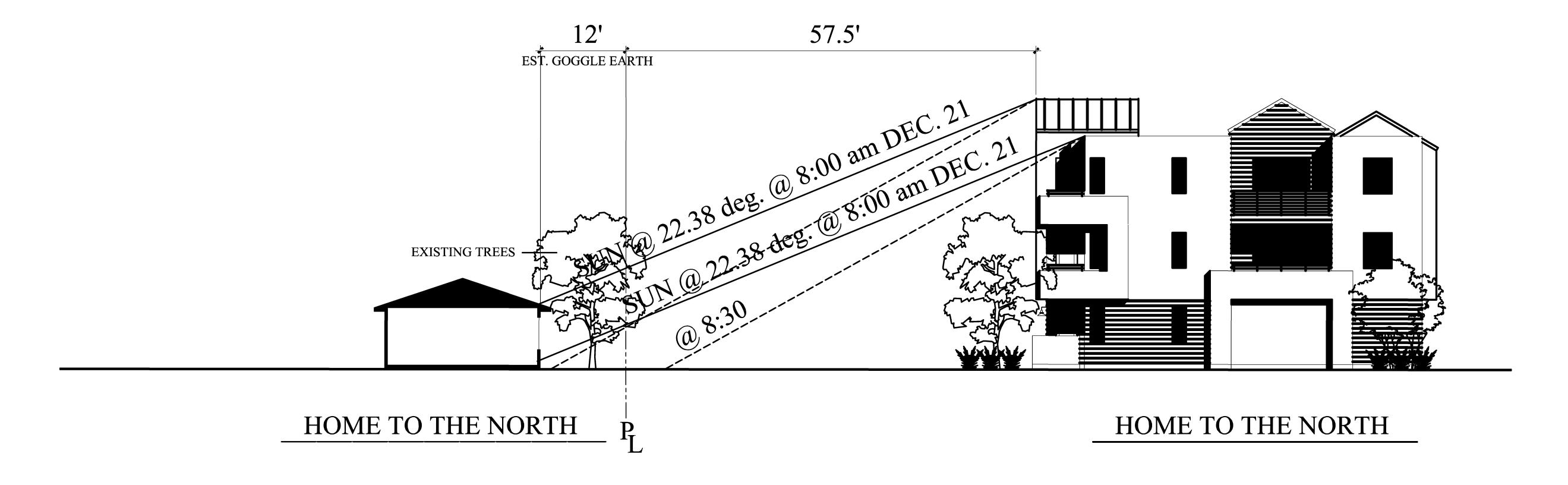
The long dimension of this building is plotted in a east west alignment.
