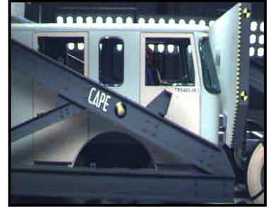
**Additional Frontal Impact:** The same cab was then struck a third time at a higher speed to impart 65,200 ft-lbs of energy into the cab (twice the ECE 29 level of energy).
