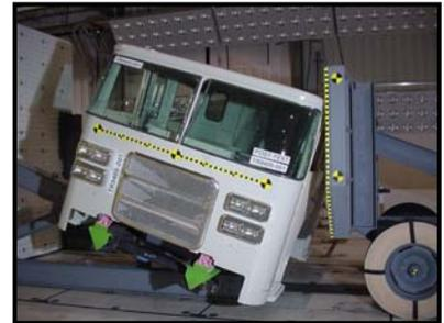
**Roof Crush:** This same test cab was then subjected to a roof crush force of 22,050 lbs. This value meets the ECE 29 criteria, which must be equivalent to the front axle rating up to a maximum of 10 metric tons.
