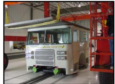
**Additional Roof Crush:** The same cab was then loaded with 60,000 lbs, 72,000 lbs, 80,000 lbs, and finally 100,000 lbs on the roof, exceeding the ECE test by 4.5 times!
