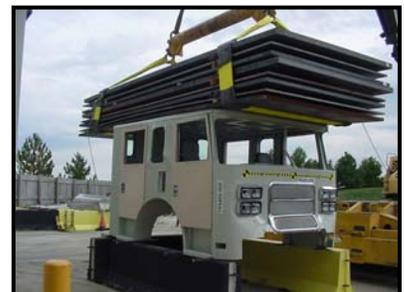
**Frontal Impact:** The test cab was struck by the 13,275 lb moving barrier at a speed sufficient to impart the required 32,600 ft-lbs of energy.
