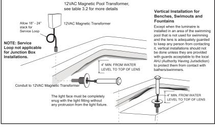
Figure 3. Standard installation with 1.5" pool wall fitting
