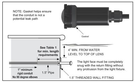
Figure 2. Standard installation with 1.5" pool wall fitting
