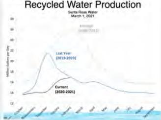
The Recycled Water Production chart represents the monthly average plant effluent flow rate from Laguna Treatment Plant.
