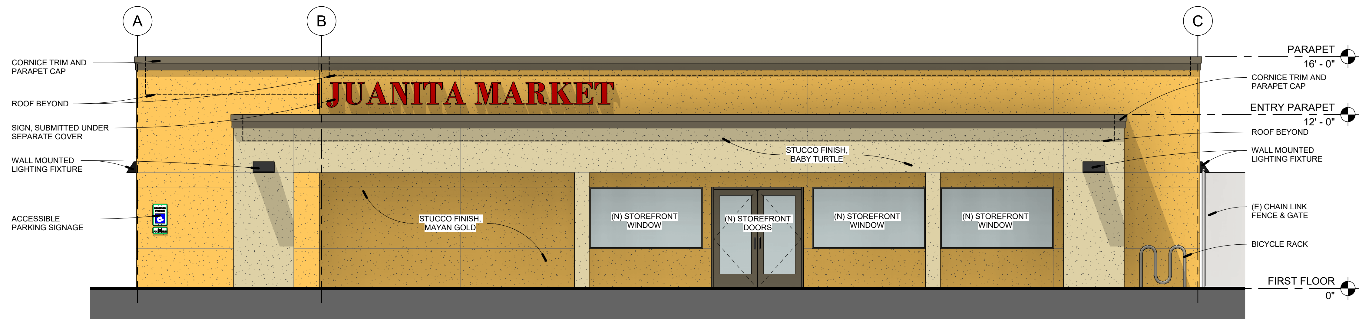
1 ELEVATION - SOUTH A103 1/4" = 1'-0"
