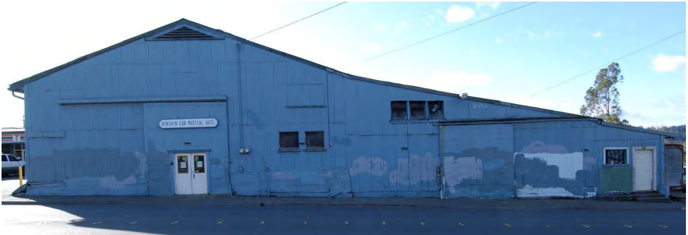
P5b. Description of Photo: East façade, looking south west across Middle Rincon Road. Notice the air vents and large rolling barn doors. These are typical features of a feed mill.
