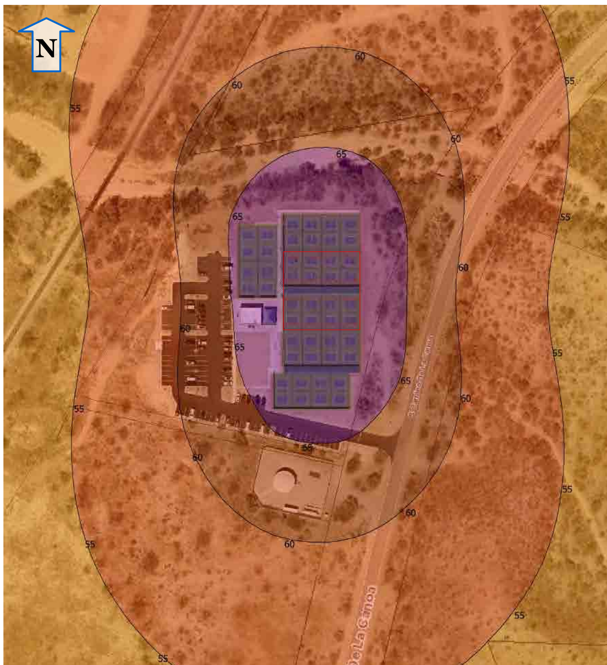
Figure 7.3. Adjusted Sound Pressure Level from Eight Pickleball Courts Aligned Laterally
