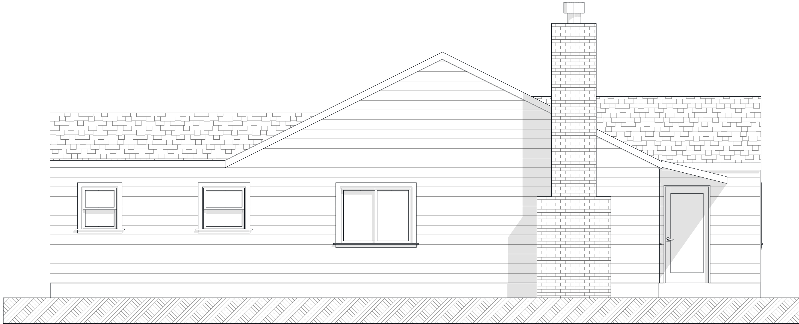
4 West Elevation (Existing) A201 SCALE: 1/4" = 1'-0"
