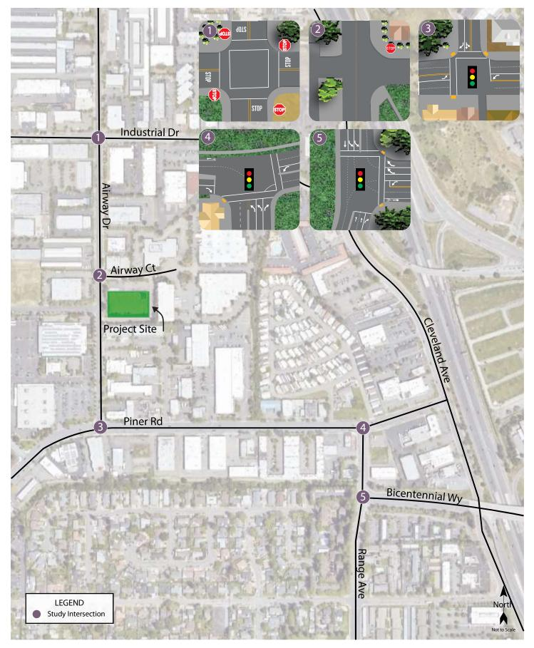
Transportation Impact Study for the Tesla Service Center Project Figure 1 – Study Area and Existing Lane Configurations
