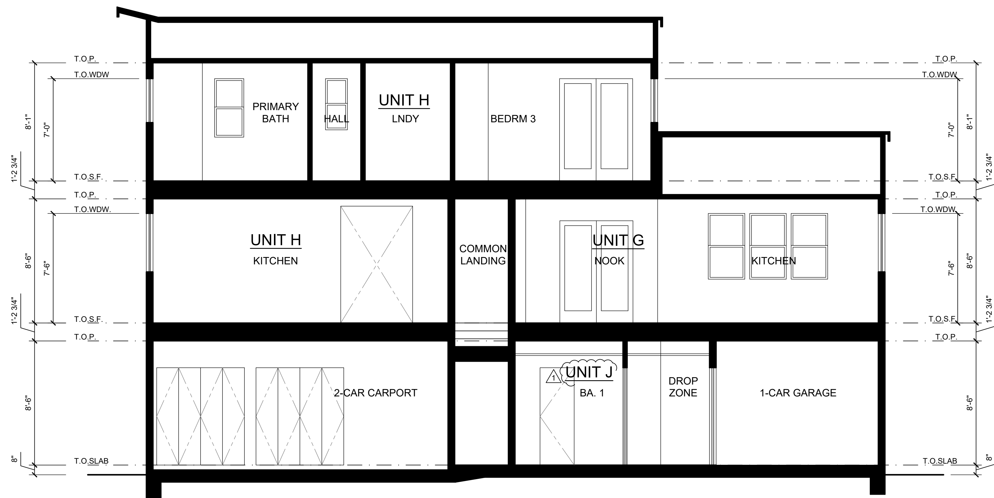
A 3-UNIT BUILDING - BUILDING SECTION A SCALE: 1/4" = 1'-0"
