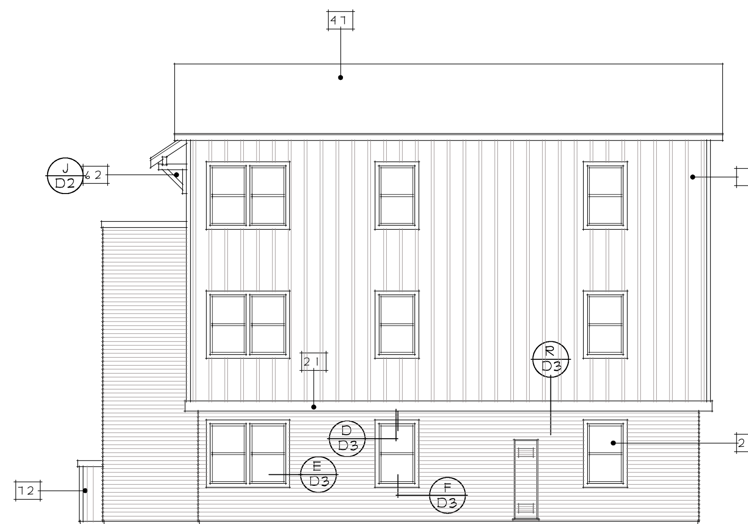
EXISTING RIGHT SIDE ELEVATION SCALE: 1/8" = 1'-0"
