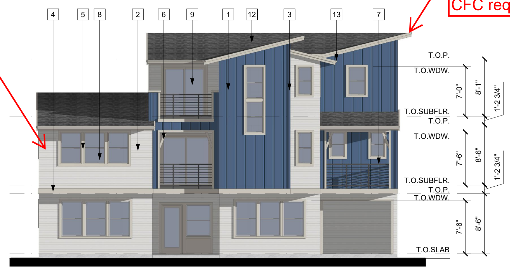
3-UNIT BUILDING - REAR ELEVATION PROPOSED SCALE: 1/8" = 1'-0"
