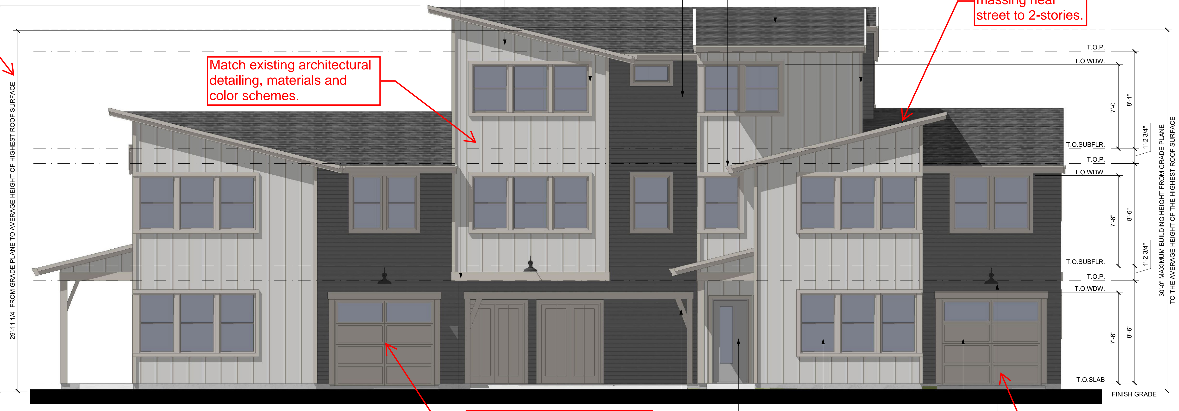
4-UNIT BUILDING - FRONT ELEVATION PROPOSED SCALE: 1/4" = 1'-0"
