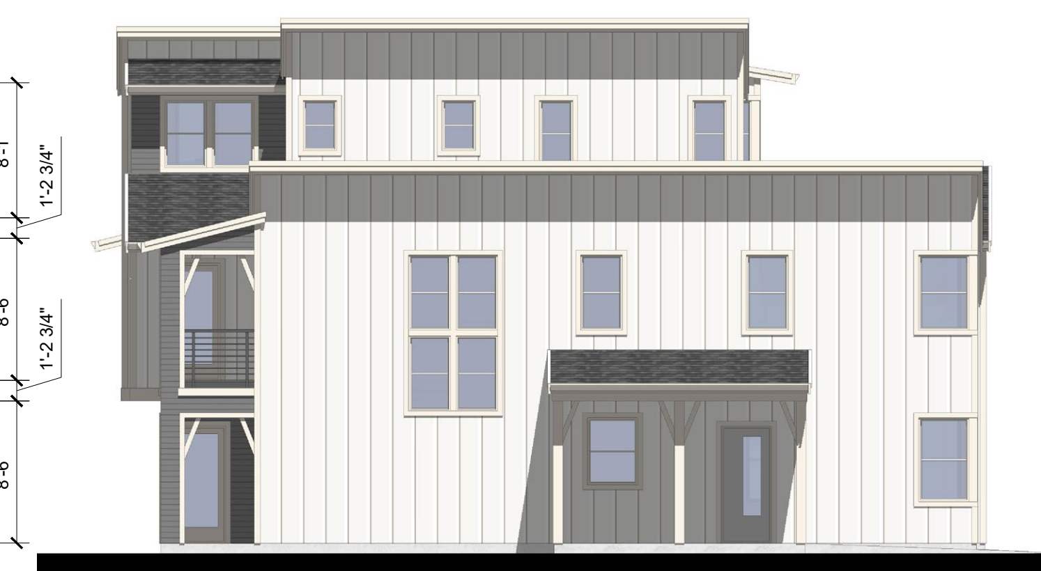
4-UNIT BUILDING - LEFT ELEVATION PROPOSED SCALE: 1/8" = 1'-0"
