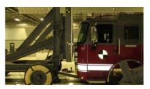
**Roof Crush:** This test cab was then subjected to a roof crush force of 110,000 lbs. This value exceeds the ECE 29 criteria, which must be equivalent to the front axle rating. This is 4.6 times higher than max. front axle rating.
