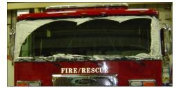
the event of breakage. The inner light will provide yet another chip resistant layer. The cab windshield will be bonded to the aluminum windshield frame using a urethane adhesive. A custom frit pattern will be applied on the outside perimeter of the windshield for a finished automotive appearance.
